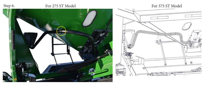
Fasten the Transfer Tube to the Talc Holding Container using the supplied exhaust clamp. Using the black hose clamp and a self tapping screw, fasten the tube to the shell assembly as shown in the image above. Tighten hardware once finished.
