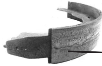
Acceptable Hairline Cracks
