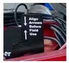
WARNING: Failure to allow locks to fully engage, as pictured below, can cause severe damage to the applicator. Look at the align arrows decal before field use.
