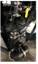
Attach the pump hydraulic hoses to the tractor so the pump operates in the lower/retract position. The pump can then be turned off in the forward "float" position. Turning the pump off in "float" instead of "neutral" allows the hydraulic system pressure to equalize and prevents the occurrence of damaging pressure spikes.
