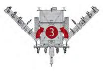
4. Main Toolbar Down (Down Pressure Circuit - Green Taped Hoses)
