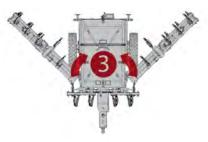
Main Toolbar Down (Down Pressure Circuit - Green Taped Hoses)
