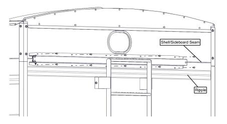
Install the Spring Return on the front of the gravity box using ten 1/4" x 3/4" self tapping bolts. Be sure the end with the cable loop is OCS. It should be positioned up against the OCS corner brace. See the chart below for model specific Spring Return locations.
