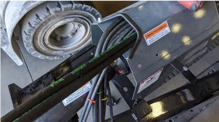
Secure the hoses with large zip ties to the grain cart as shown.
