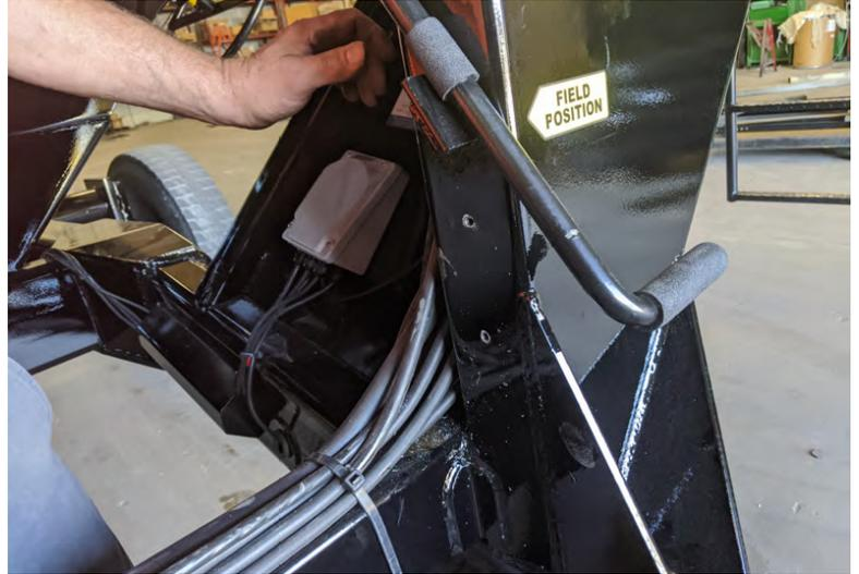
Attach mount using the two 1/4" x 3/4" bolts and 1/4" serrated flange nuts.
