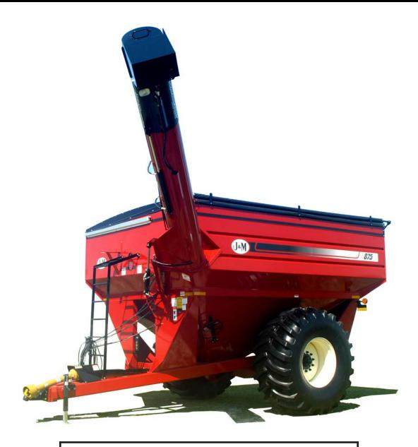
Extend the auger into the unload position. Engage the upper auger into the lower auger by rotating the driveline.
