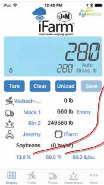
Unload one load from the grain cart. The Moisture and Temperature will update after every reading (1 per second) Remember the moisture and temperature readings. Note: You must select the correct type of commodity in the field section for accurate readings. If you see a very low reading this would be the first thing to check.
