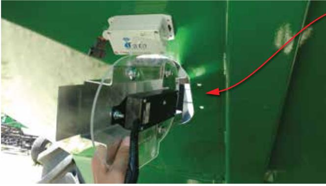
Insert the fully assembled Moisture mount through the window hole.
