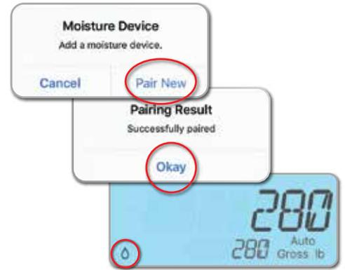
Press "Pair New". It will now pair with the closest iFarm Moisture Sensor. Press Okay to confirm pairing. At the display tab a new icon will appear. This Water Drop Moisture icon indicates you are currently connected to the iFarm Moisture Sensor.
