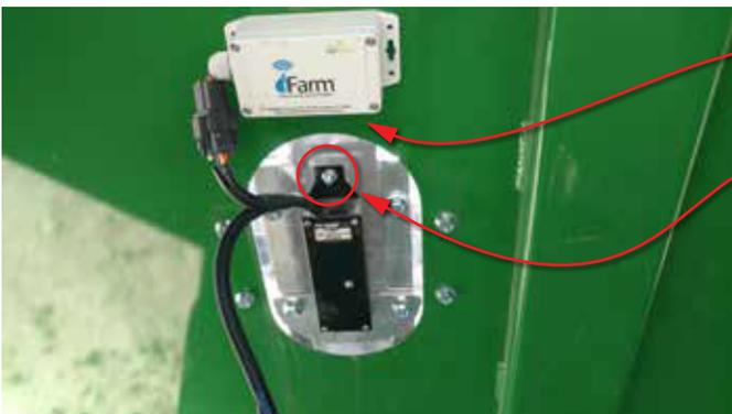
Attach the gray iFarm moisture unit on top of the front window about three inches above.
