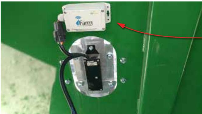
Using the power cable you removed from the top tube conduit, reattach it to the AgLeader sensor and connect the iFarm Unit to the AgLeader unit.
