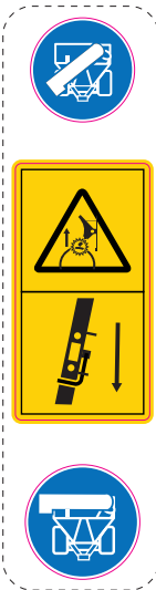
When Moving Auger Tube from Storage Position to Field Position, Ensure Auger Rest is in Field Position. Damage to the Tube Can Occur if Auger Rest is in Storage Position During the Process.
