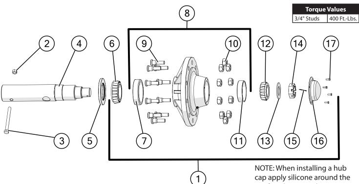
cap apply silicone around the rim for a better seal.
