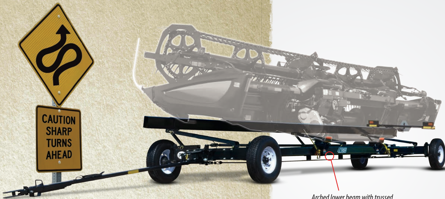
Arched lower beam with trussed understructure for maximum support.
